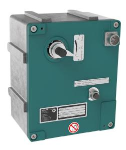
motors disk nevertheless quick response times can be gained. In case of voltage loss a return spring ensures setting back to zero position. Optionally the actuator is available without return spring. A contactless feedback system is integrated onto the governors output shaft offering an electrical position signal to any external control unit.
