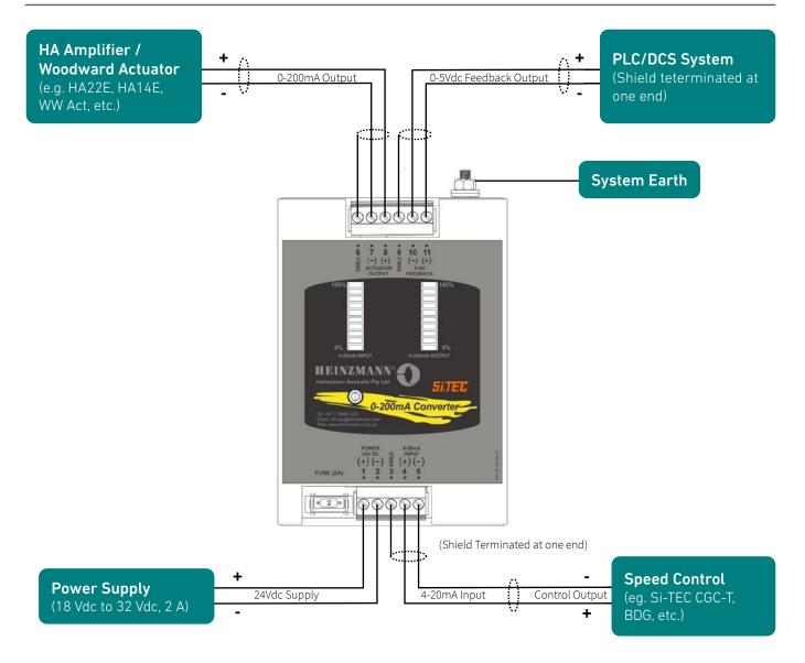
The signal converter is internal panel flush mounted with 2 x M6 mounting screws required.
